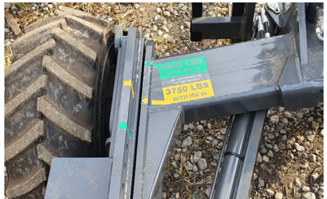
Mast Capacity at FULL REACH (Yellow Arrows aligned) Lift Capacity 1700kg / 3750lb
