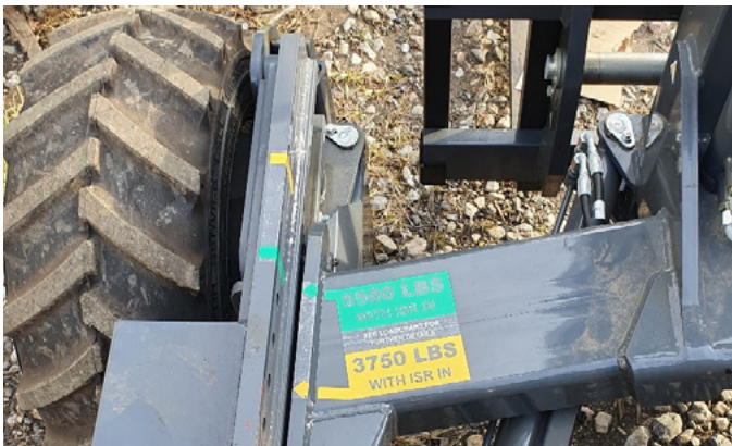
Mast Capacity at OPTIMUM REACH (Green Arrows aligned) Lift Capacity 2500kg / 5500lb
